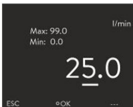
Fig. 50: Setting the flow rate set point
