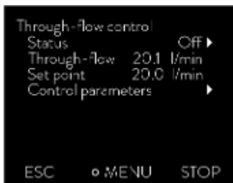
Fig. 49: Through-flow control menu
